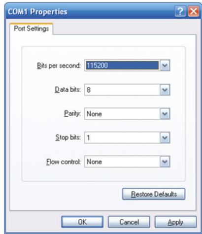
**Figure 5-2:** COM Port Configuration
