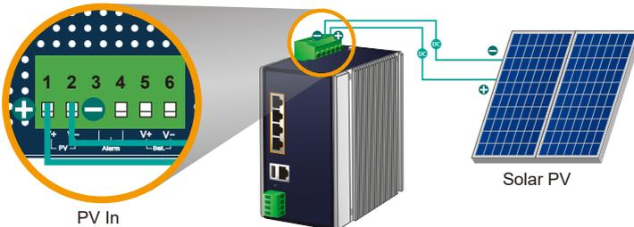
1. Connect the **negative electrode of the PV panel** to the terminal for the **negative electrode of the PV panel on the BSP-360**.
