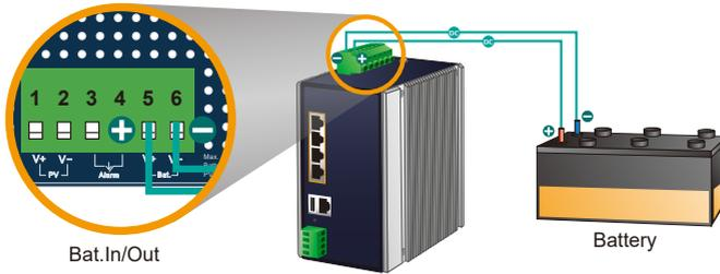
1. Connect the **negative electrode of the battery** to the terminal for the **negative electrode of the battery on the BSP-360**. By default, the lithium battery is in use.
