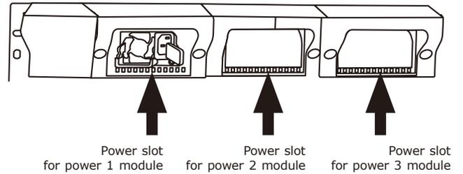
Figure 1. Power slots of CS-6306R
