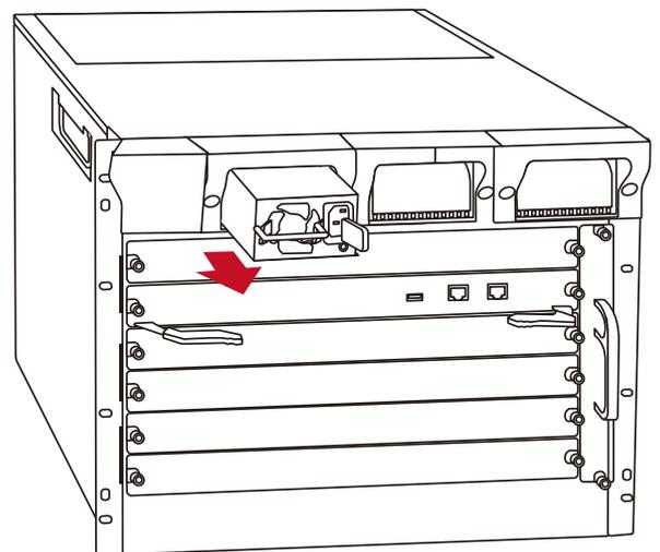
**Figure 3.** Installing/removing the CS6-PWR550-AC
