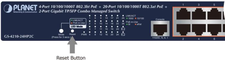
Figure 5-4: GS-4210-24HP2C Reset Button
