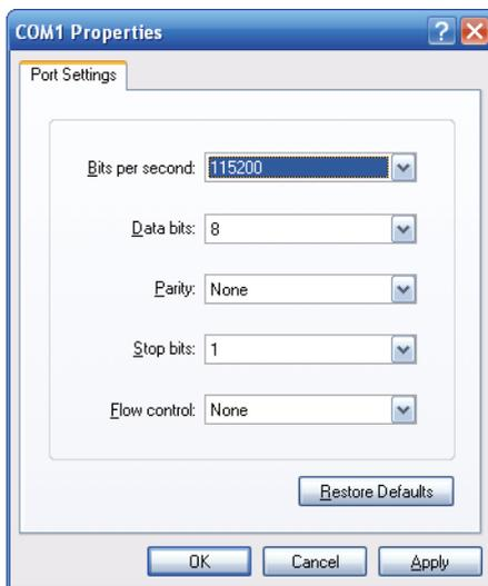
**Figure 3-2:** COM Port Configuration
