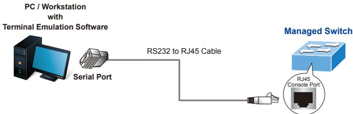
**Figure 3-1:** L2+ Managed PoE+ Switch Console Connectivity
