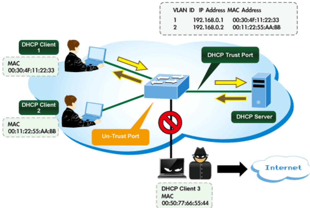
Configure DHCP Snooping on this page. The DHCP Snooping Configuration screen in [Figure 4-5-6](#) appears.
