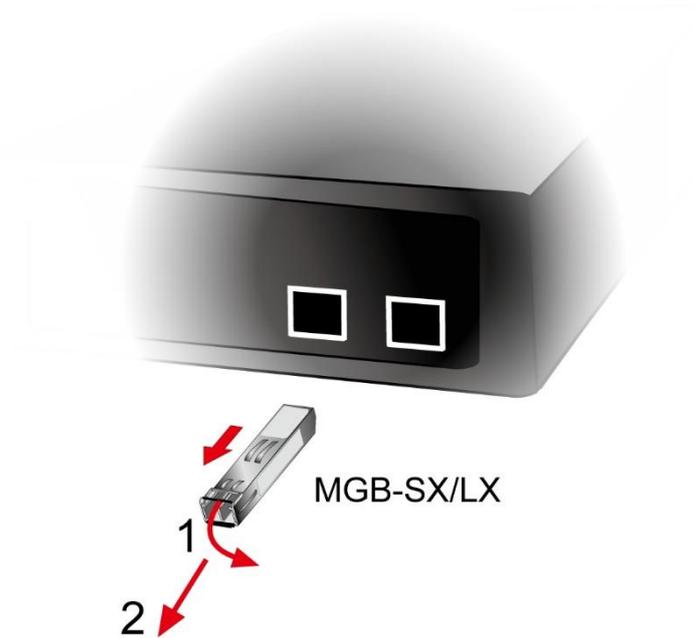
**Figure 2-2-5:** How to Pull Out the SFP/SFP+ Transceiver
