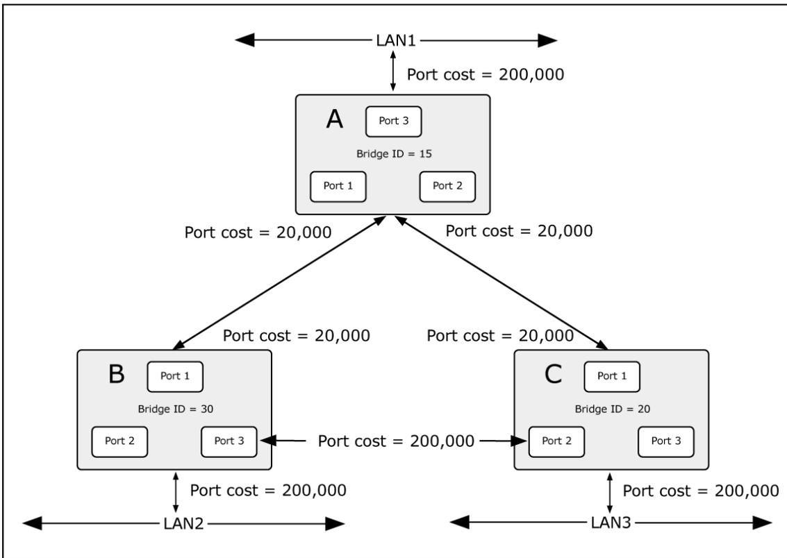
Figure 4-3-4-2: Before Applying the STA Rules
