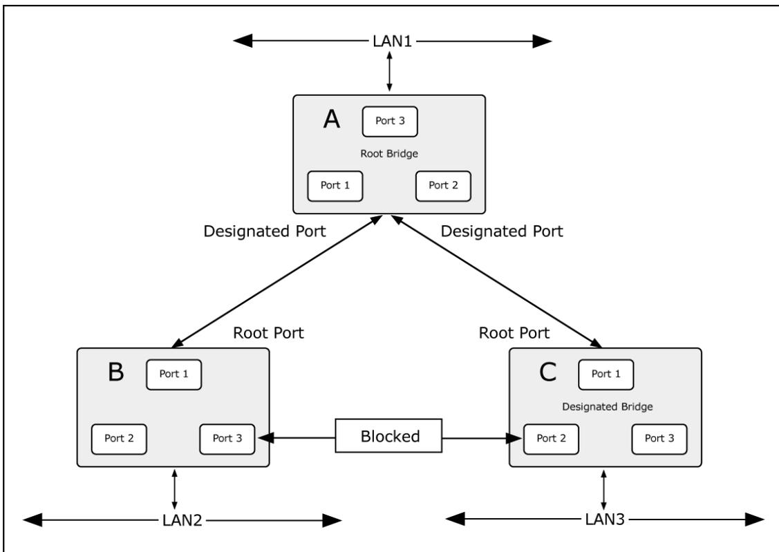
Figure 4-3-4-3: After Applying the STA Rules
