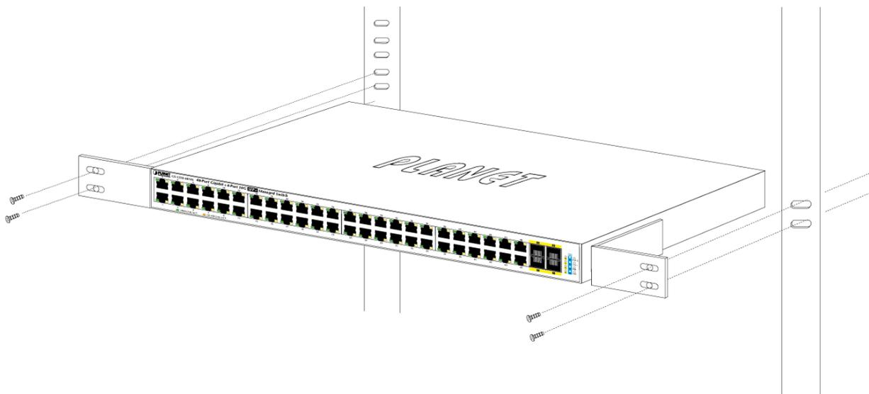
Figure 2-2-3: Mounting Managed Switch in a Rack
