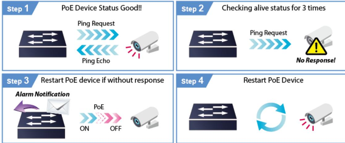
This page provides you with how to configure PD Alive Check. The screen in Figure 4-6-7 appears.
