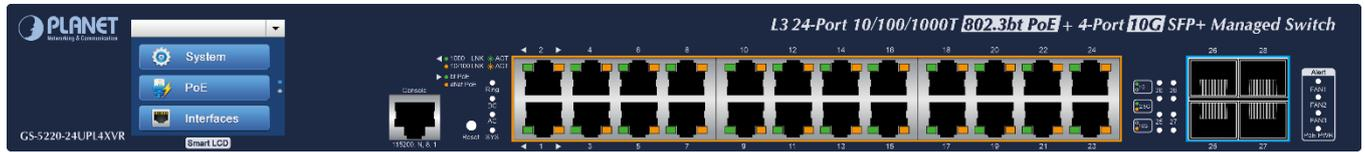
Figure 2-1-3: Front Panel of GS-5220-24UPL4XVR
