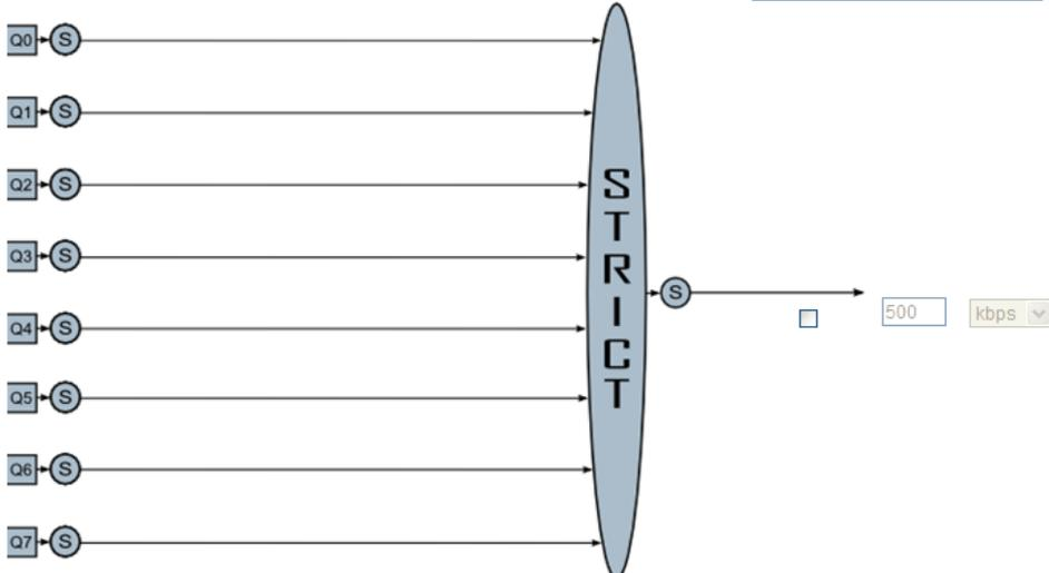
The diagram illustrates the data flow from eight queues (Q0 through Q7) into a central vertical oval labeled "STRICT". Each queue is represented by a small circle with an "S" and an arrow pointing towards the "STRICT" oval. From the right side of the "STRICT" oval, an arrow points to a "Port Shaper" section, which includes a rate of 500 kbps and an "Enable" checkbox.
