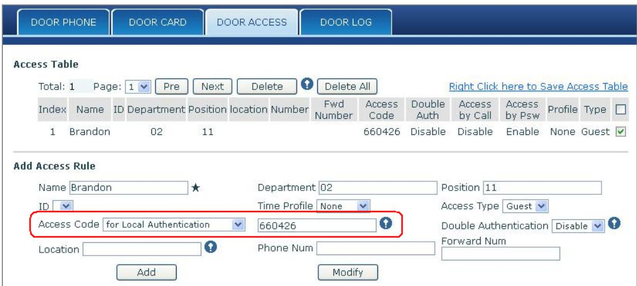
The screenshot shows the 'Access Table' and 'Add Access Rule' sections. The 'Add Access Rule' form has the 'Access Code' field highlighted with a red box. The form includes fields for Name, Department, Position, ID, Time Profile, Access Type, and Double Authentication.
