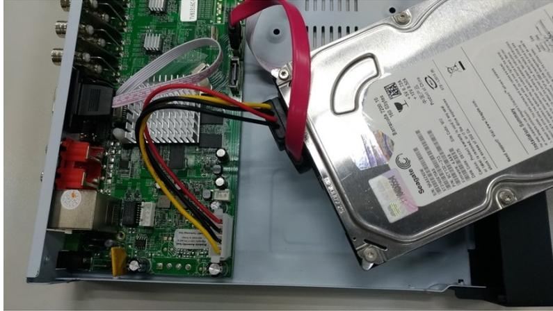
3. Please align the screw holes on the HDD with those on the HDVR case and secure them with the given screws.
