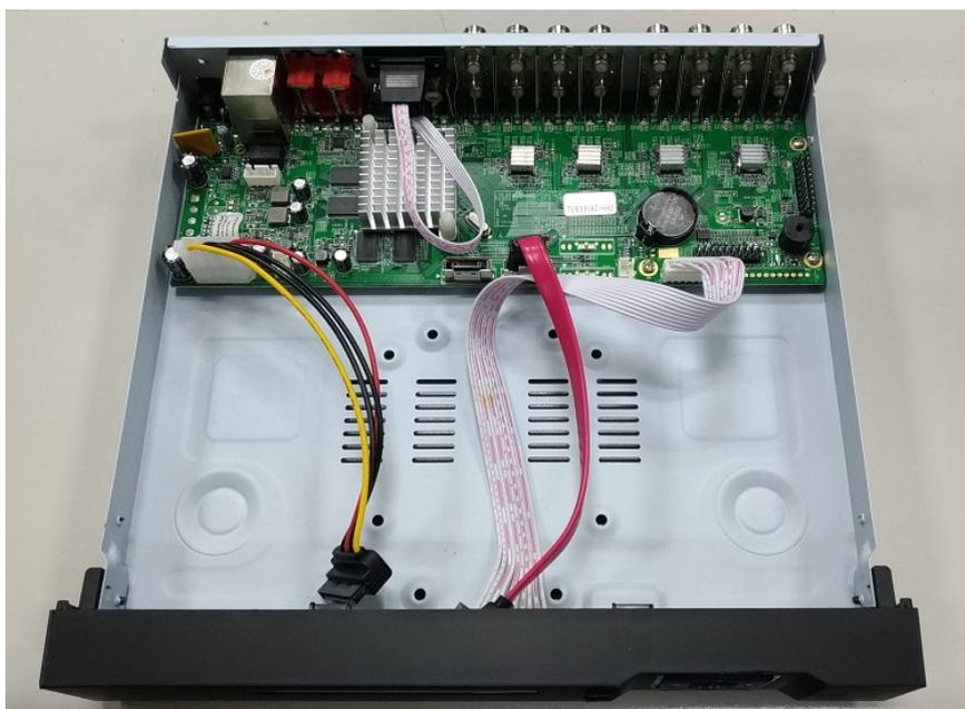
2. Plug the HDD power cable and SATA cable into the slots of the PCBA board and the HDD, respectively, making sure the connections are well done.
