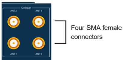
**Step 2:** Fasten the 5G NR antenna extenders to the connectors.
