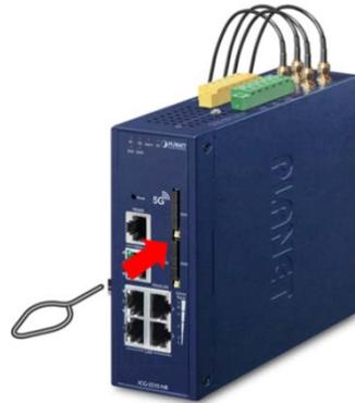
B. Pull out the tray gently from the tray slot. Place the SIM card on the tray with the gold-colored contacts facing upwards.
