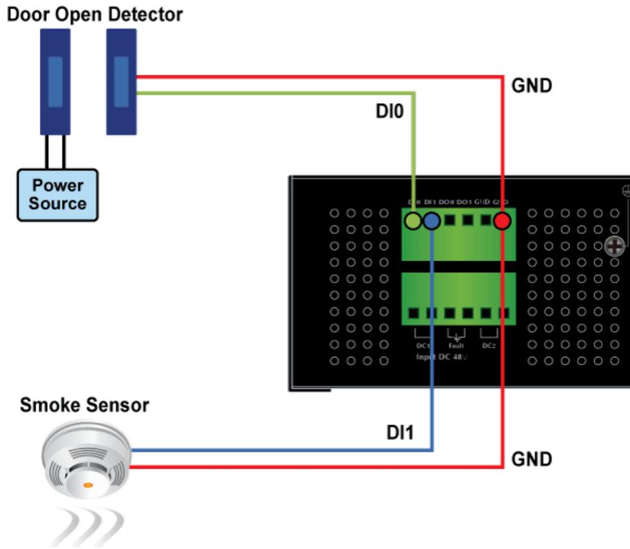
Figure 2-7: Wiring DI0 and DI1 to Open Detector
