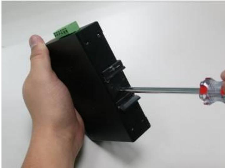
**Step 2:** Lightly slide the DIN-rail bracket into the track.
