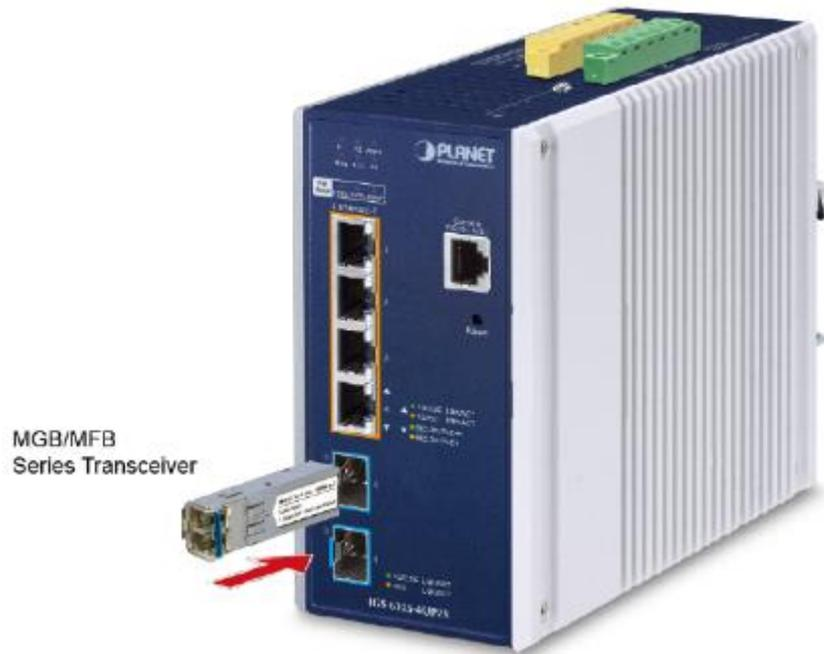
Figure 2-9: Plugging in the SFP Transceiver
