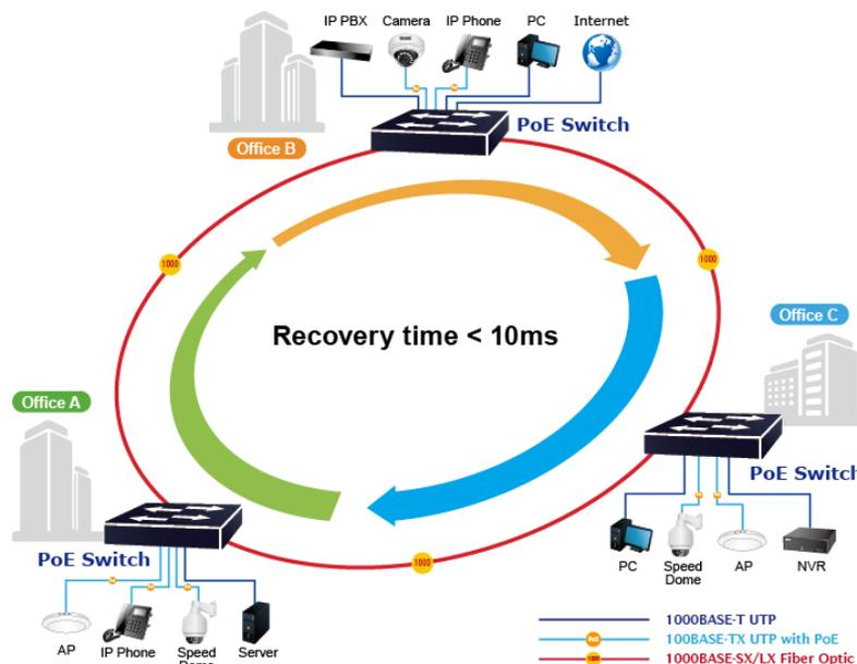
**Figure 4-8-1: Ring Example Diagram**
