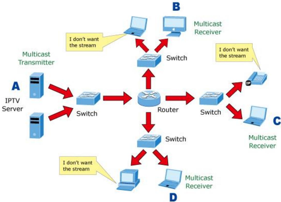
Figure 4-3-5-2: Multicast Flooding
