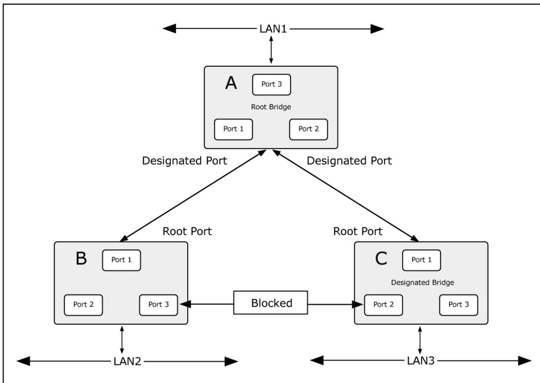
**Figure 4-3-4-3:** After Applying the STA Rules
