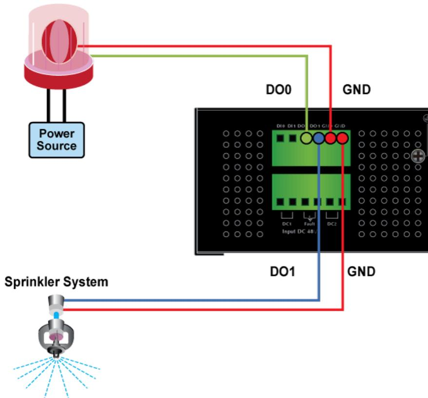
Figure 2-8: Wiring DO0 and DO1 to Open Detector
