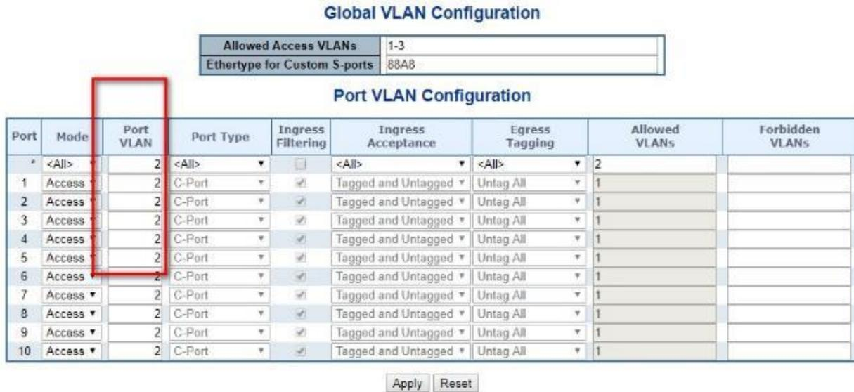
**Figure 4-3-3-13:** Changes Port VLAN of Port 1~3 to be VLAN2 and Port VLAN of Port 4~6 to be VLAN3
