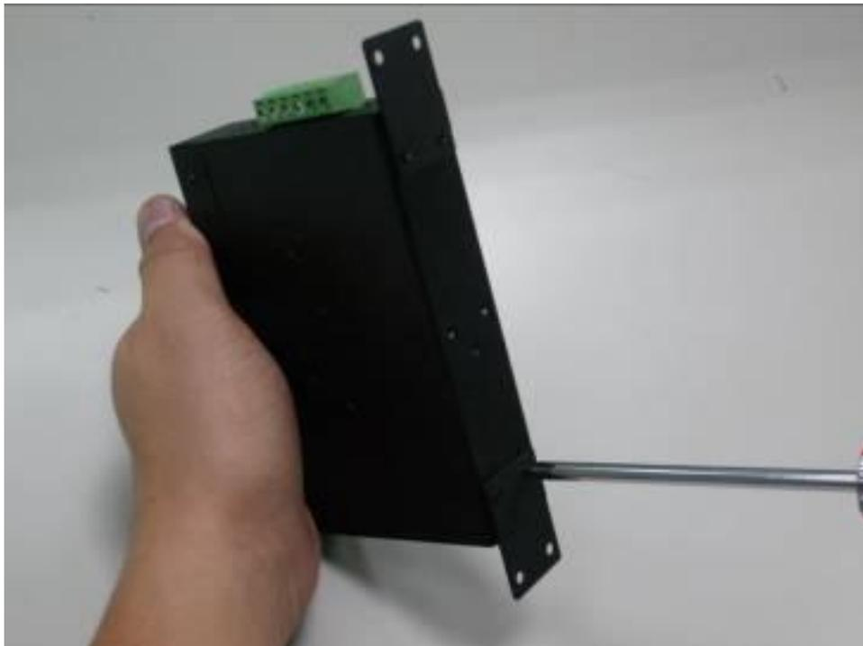
**Step 3:** Use the screwdriver to screw the wall mount plate on the **Industrial Managed PoE+ Switch**.
