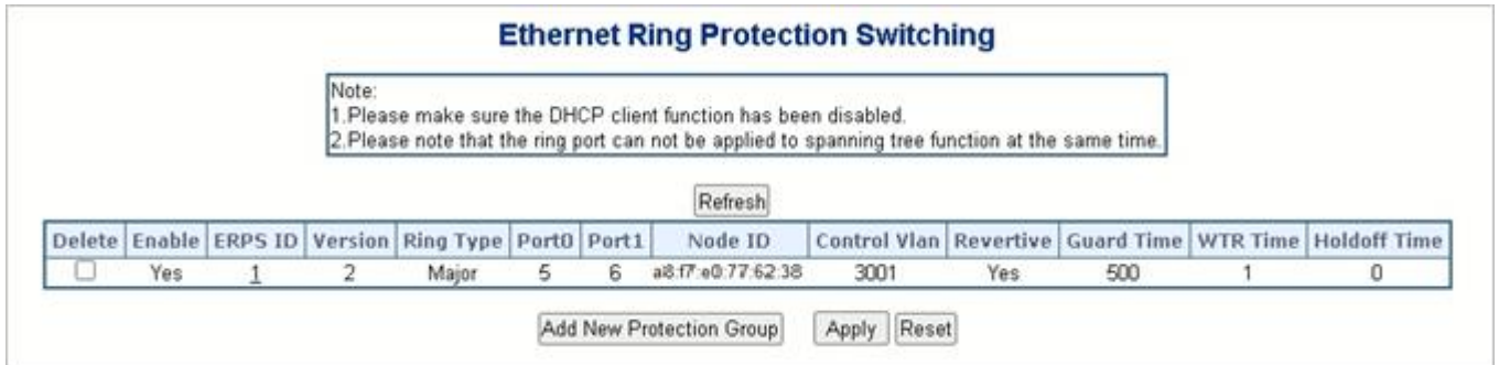
Figure 4-14-2: Ethernet Ring Protection Switching page screenshot
