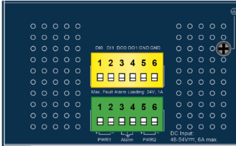
Figure 2-12: IGS-5225-8P2T2S, IGS-5225-8P2T4S, IGS-5225-8P4S and IGS-5225-8P4S-12V Upper Panel
