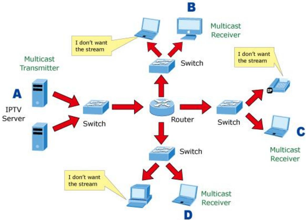
Figure 4-3-10-2: Multicast Flooding
