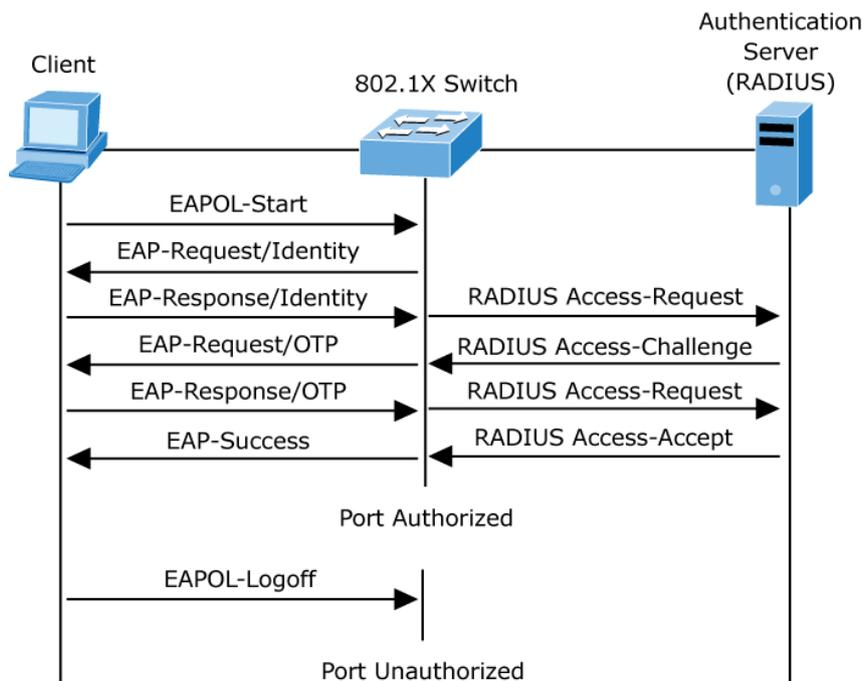
Figure 4-5-2-2: EAP Message Exchange
