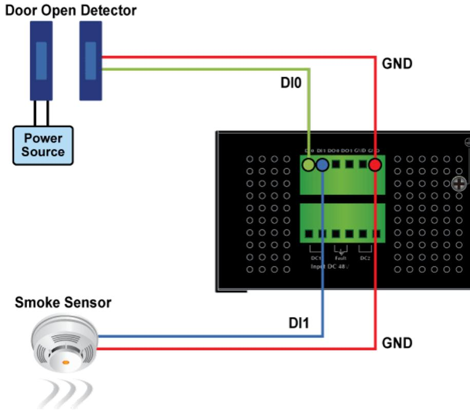
Figure 2-19: Wiring DI0 and DI1 to Open Detector
