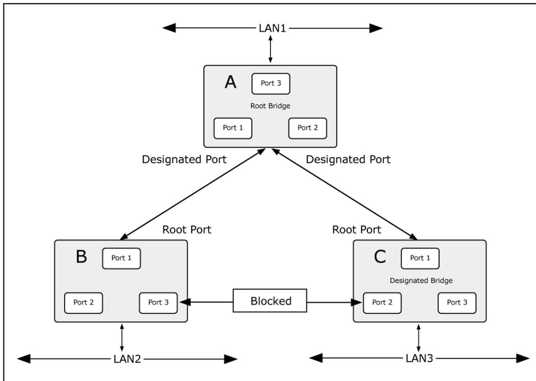
**Figure 4-3-9-3:** After Applying the STA Rules
