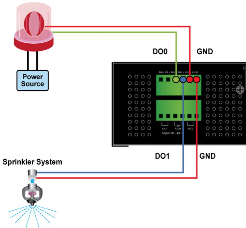
Figure 2-20: Wiring DO0 and DO1 to Open Detector
