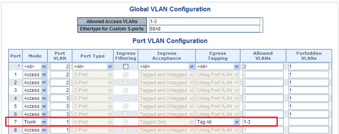
**Figure 4-3-3-14:** VLAN Overlap Port Setting & VLAN 1 – The Public Area Member Assign
