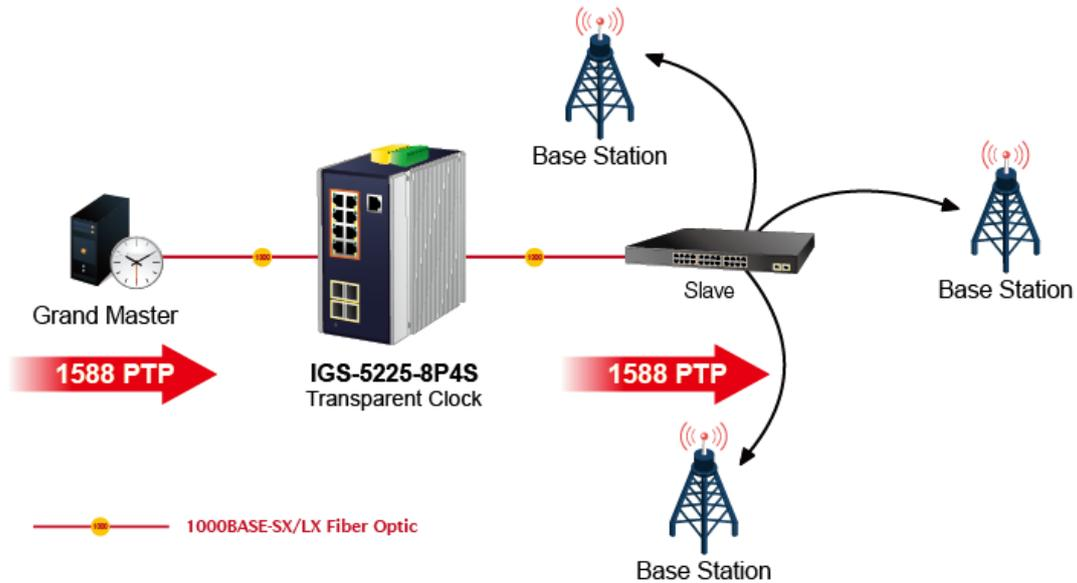
PTP was originally defined in the **IEEE 1588-2002** standard, officially entitled "*Standard for a Precision Clock Synchronization Protocol for Networked Measurement and Control Systems*" and published in 2002. In 2008 a revised standard, **IEEE 588-2008** was released. This new version, also known as PTP Version 2, improves accuracy, precision and robustness but is not backwards compatible with the original 2002 version.
