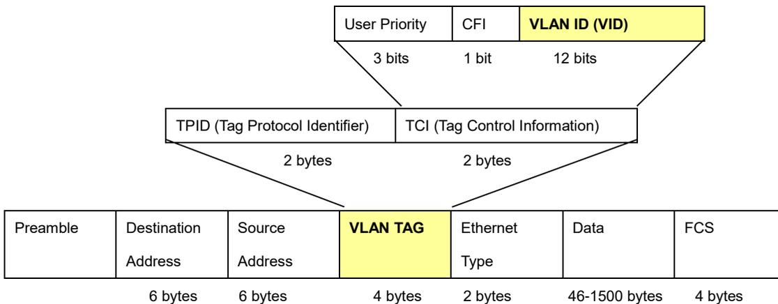
The Ether Type and VLAN ID are inserted after the MAC source address, but before the original Ether Type/Length or Logical Link Control. Because the packet is now a bit longer than it was originally, the Cyclic Redundancy Check (CRC) must be recalculated.
