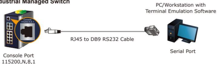
A terminal program is required to make the software connected to the Industrial Managed Switch.
