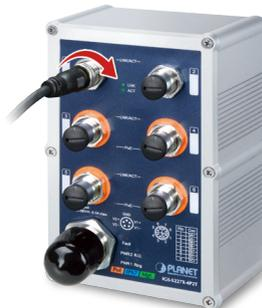
**Step 4:** Insert the M23 power female connector into the M23 male port of the power input.
