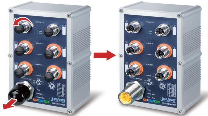
**Step 2:** Insert the M12 UTP male connector into the M12 female Gigabit Ethernet port of the Industrial Managed PoE+ Switch.
