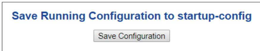
3. Or the other way to save the setting is to Click **Maintenance, Switch Maintenance, Save Startup Config**.
