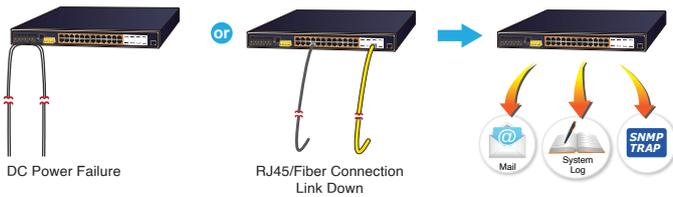
**Digital Input and Digital Output for External Alarm**
