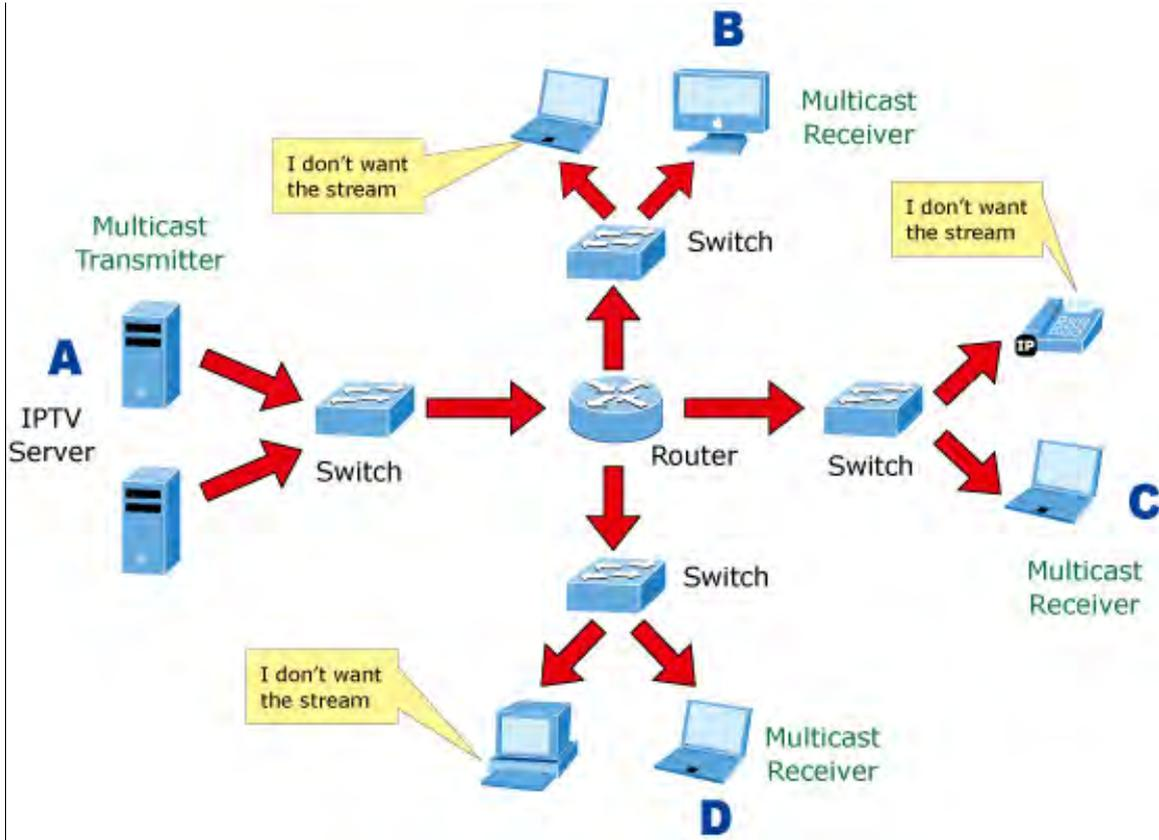
Figure 4-3-9-2: Multicast Flooding
