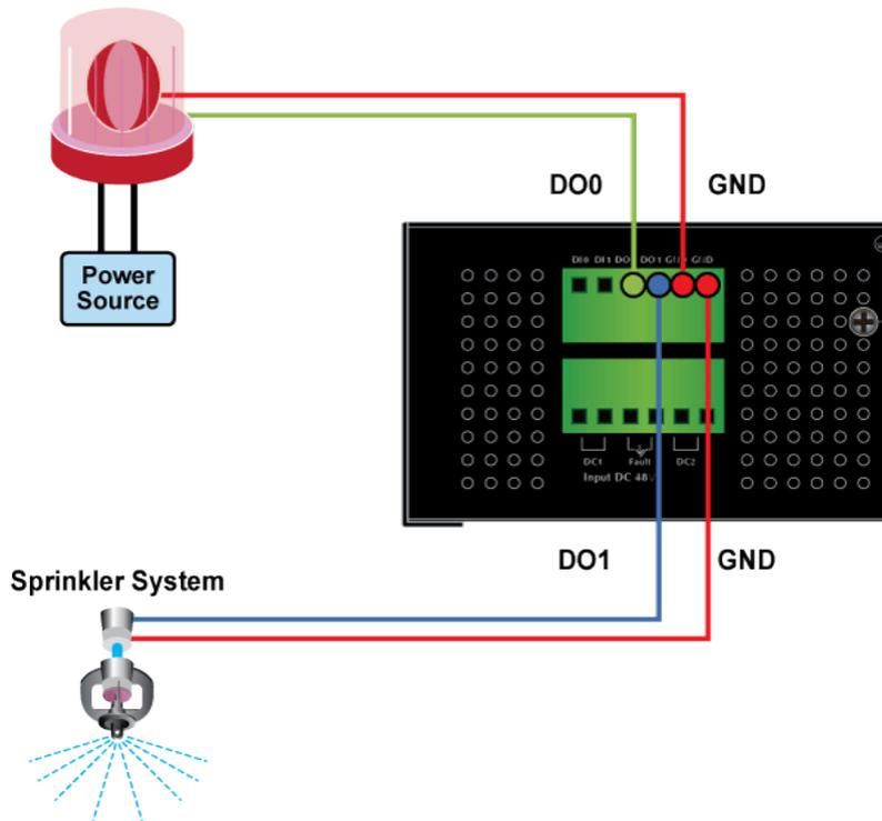
Figure 2-1-25: Wires DO0 and DO1 to Open Detector
