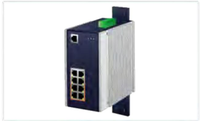
**Step 3:** Use the screwdriver to screw the wall-mount plate on the **Industrial Managed Switch**.
