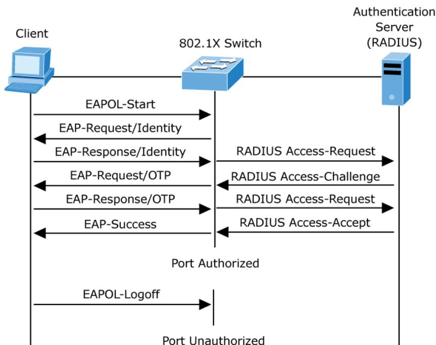
Figure 4-5-2-2: EAP Message Exchange
