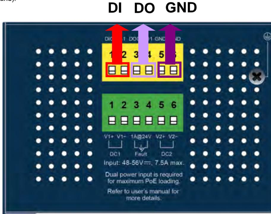
Figure 2-1-22: Wiring the DI and DO of IGS-6325 Din-rail Series.
