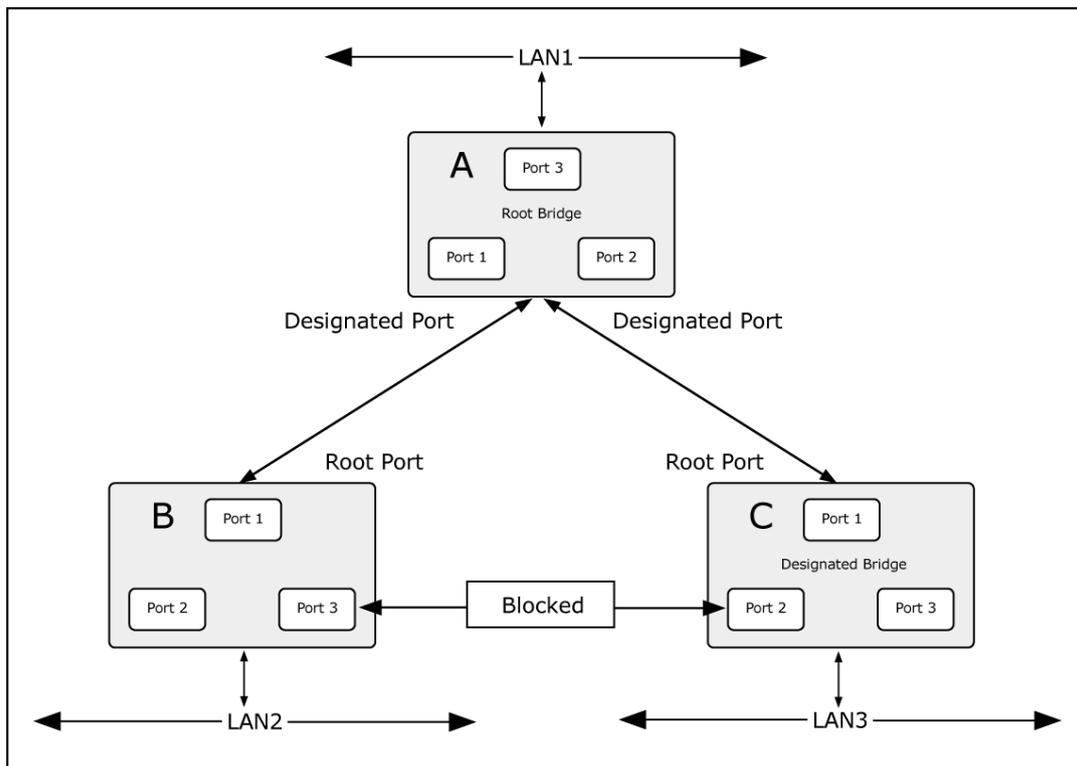
Figure 4-3-8-3: After Applying the STA Rules
