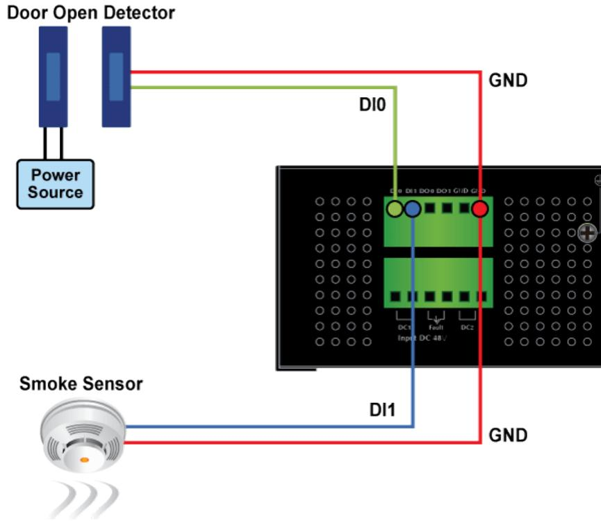
Figure 2-1-24: Wires DI0 and DI1 to Open Detector
