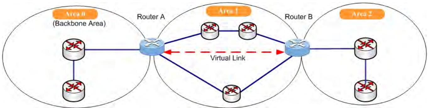
Following is OSPF virtual link configuration table. The virtual link is established between 2 ABRs to overcome that all the areas have to be connected directly to the backbone area. The screen in [Figure 4-10-4-8](#) appears.
