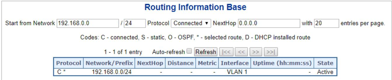
**Figure 4-10-3:** IPv4 Routing Information
