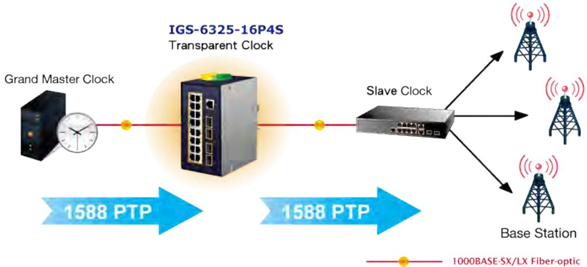
PTP was originally defined in the **IEEE 1588-2002** standard, officially entitled "*Standard for a Precision Clock Synchronization Protocol for Networked Measurement and Control Systems*" and published in 2002. In 2008 a revised standard, **IEEE 588-2008** was released. This new version, also known as PTP Version 2, improves accuracy, precision and robustness but is not backwards compatible with the original 2002 version.
