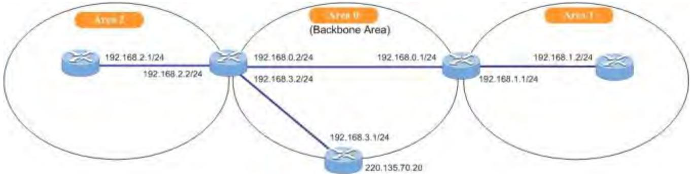
Following is OSPF area configuration table. It is used to specify the OSPF enabled interface(s). When OSPF is enabled on the specific interface(s), the router can provide the network information to the other OSPF routers via those interfaces. The screen in [Figure 4-10-4-2](#) appears.
