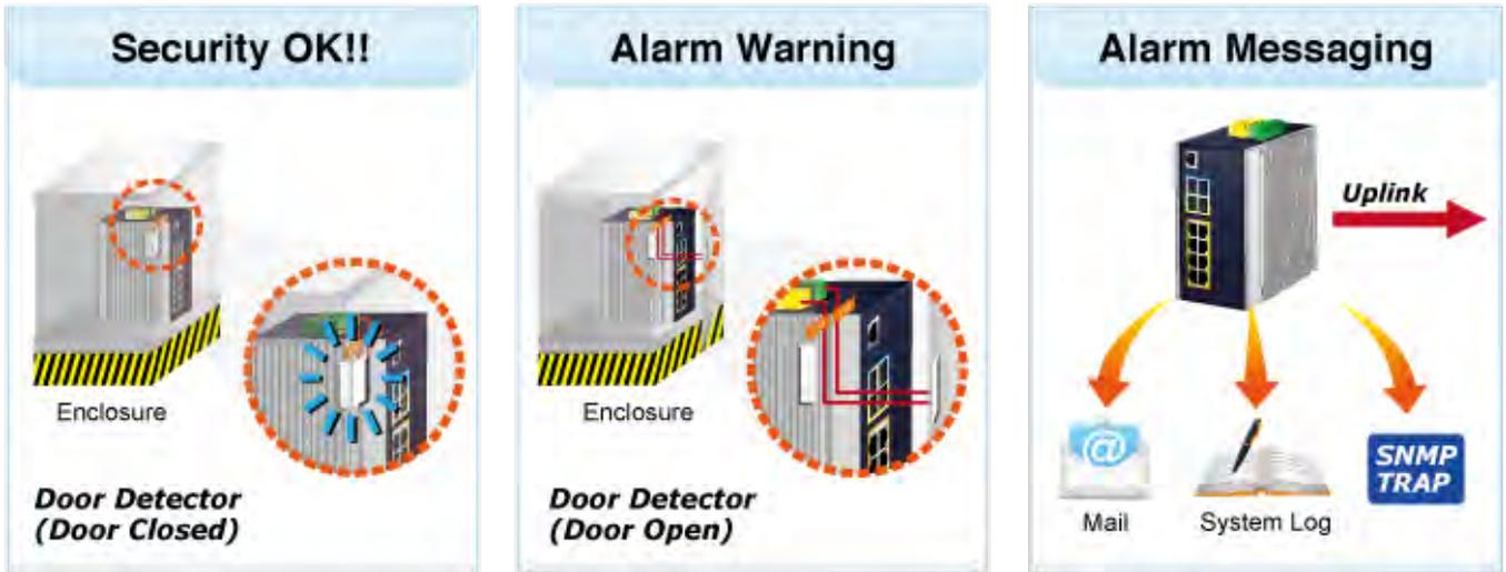
**Digital Output** allows user to monitor the switch port and power, and let system issue a high or low signal to an external device (such as alarm) when the monitor port or power has failed.
