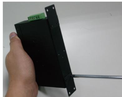
Figure 5-4: Placing Wall-mount Plate on Industrial Device
