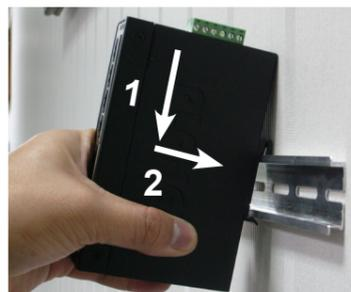
Figure 5-1: DIN-rail mounting
