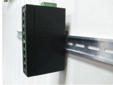
Figure 5-2: Complete DIN-rail mounting
