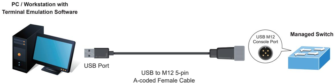
**Figure 7-1:** Industrial Managed Switch Console Connectivity
