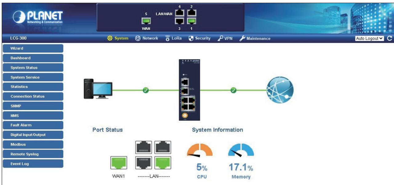
**Figure 4-4:** Web-based Main Screen of LoRaWAN Gateway
