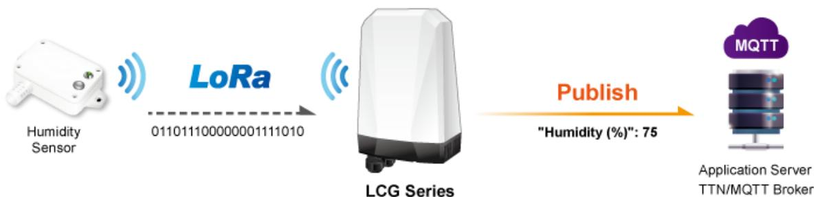
Additionally, the built-in MQTT broker in the LCG-300 series facilitates data parsing and collection, enabling users to obtain data quickly and conveniently. This is possible both through the internal MQTT broker and an external MQTT broker. This functionality helps reduce the costs associated with building network servers and minimizes the complexity of the network architecture.
