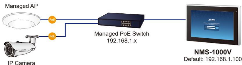
**Step 2. Switch:** Log in to the switch’s Web user interface and **enable** the **SNMP and LLDP** function.
