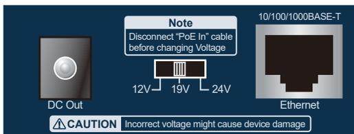
2. Connect standard UTP cable from "Ethernet" port of the POE-172S to remote device.
