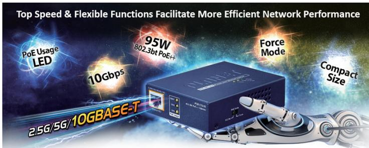
The POE-176-95, adopting the IEEE 802.3bt standard, instead of delivering power over 2-pair twisted UTP – be it end-span (Pins 1, 2, 3 and 6) or mid-span (Pins 4, 5, 7 and 8), provides the capability to source up to 95 watts of power by using all the four pairs of standard Cat. 5e/6 Ethernet cabling. In the new 4-pair system, it can offer more PoE applications, such as:
