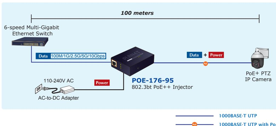
*Installation of 802.3bt PoE Injector and Splitter*
