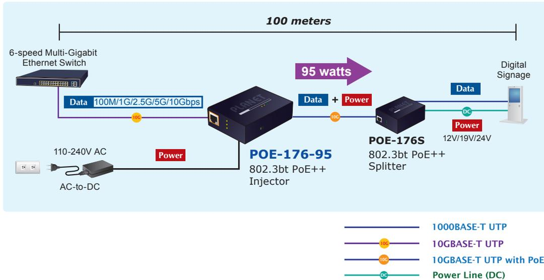
*Extended Installation of IEEE 802.3bt Injector and PoE Network*
