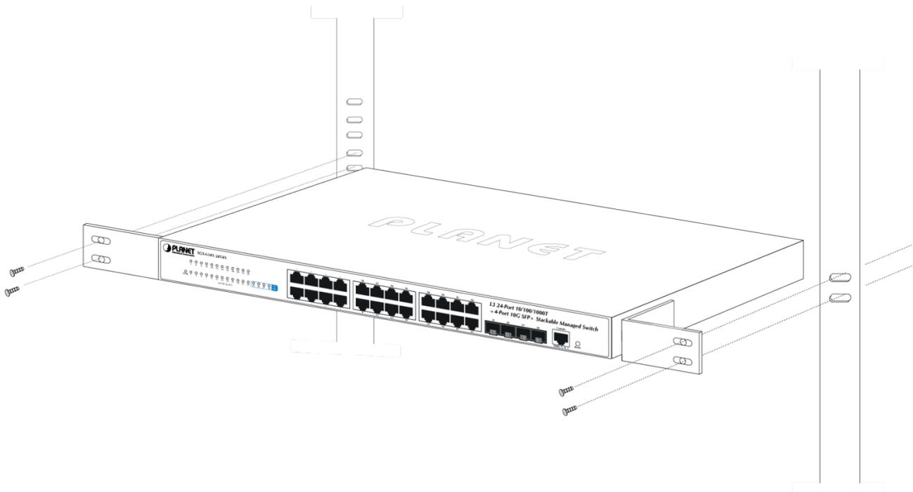
**Figure 2-2-3** Mounting SGS-6341 Series in a Rack
