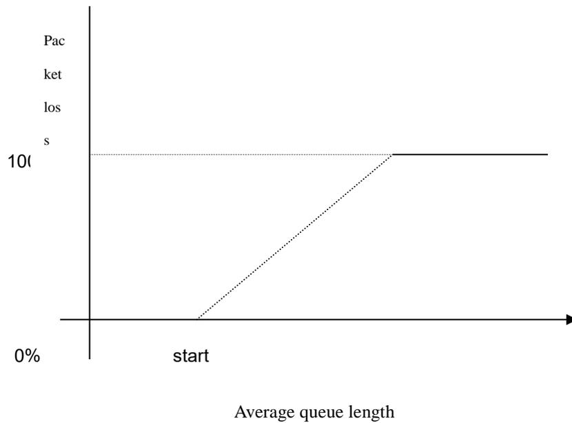
When the queue length is less than **start**, packets will not be dropped.
