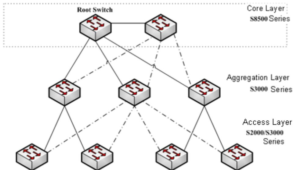
Figure 1.2 Switching network topology
