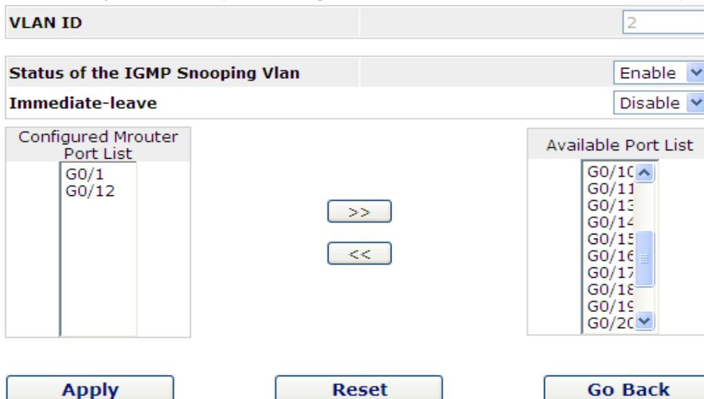
The screenshot shows the configuration page for a new IGMP Snooping VLAN with the following details:
