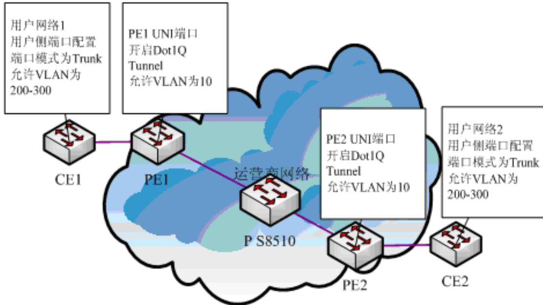
Figure 4 Typical configuration of Dot1Q tunnel
