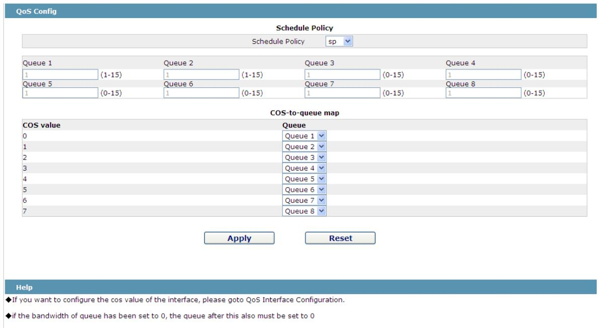
The screenshot shows the 'QoS Config' interface. At the top, there is a 'Schedule Policy' dropdown menu set to 'sp'. Below this, there are eight queues arranged in two rows of four. Each queue has a 'Weight' input field (all set to '1') and a 'Bandwidth' input field (all set to '(0-15)').
