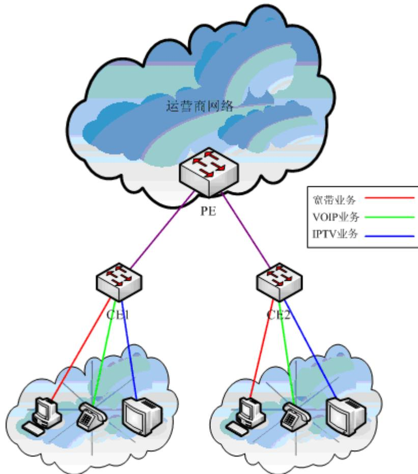
Figure 8 Typical configuration of Dot1Q tunnel (3)
