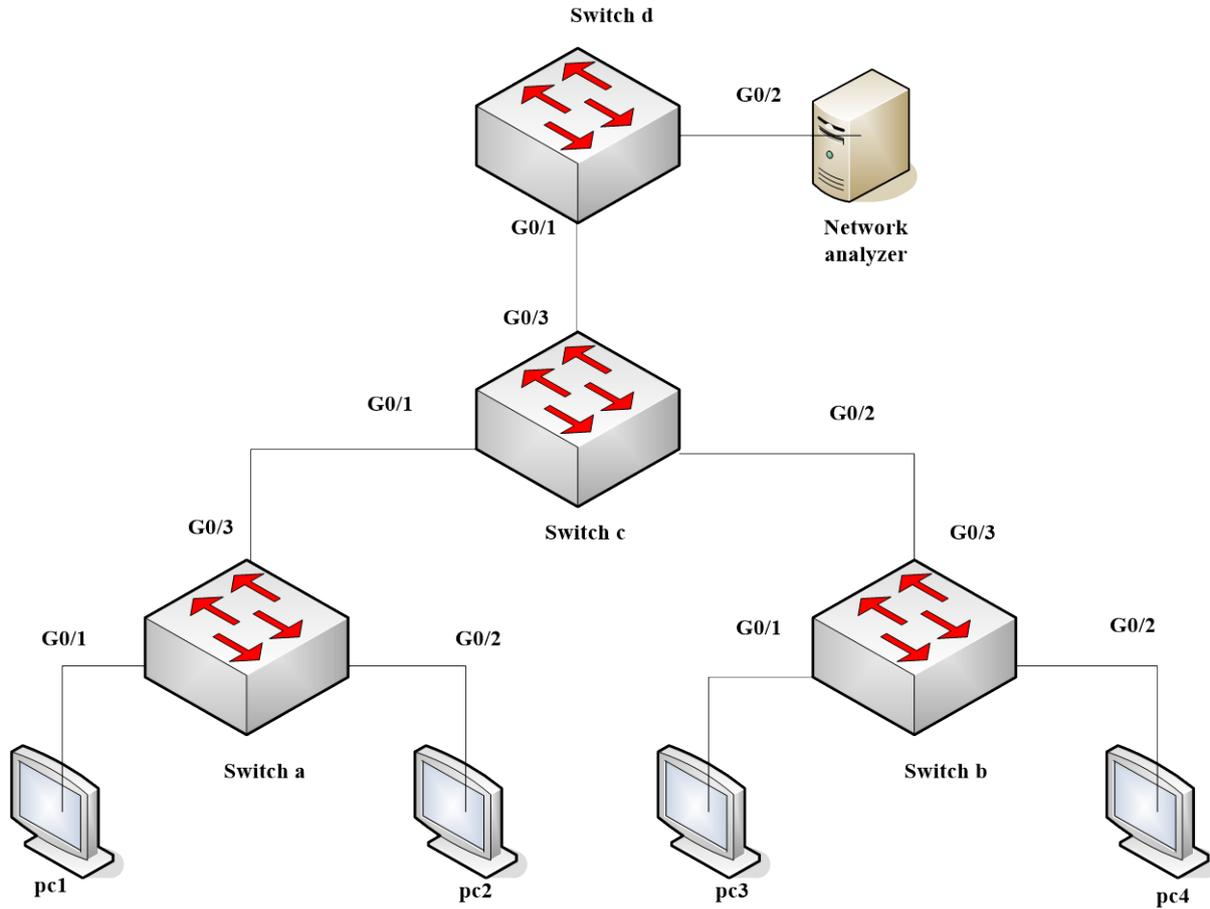
You need to monitor the traffic of interface g0/1 on switch a and interface g0/1 on switch b by the network analysis meter.
