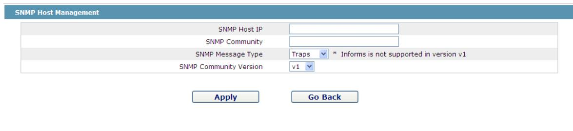
The screenshot shows the 'SNMP Host Management' configuration page. It features a form with four input fields: 'SNMP Host IP', 'SNMP Community', 'SNMP Message Type' (dropdown menu set to 'Traps' with a note '\* Informs is not supported in version v1'), and 'SNMP Community Version' (dropdown menu set to 'v1'). Below the form are two buttons: 'Apply' and 'Go Back'.
