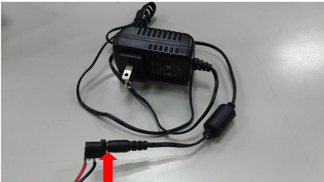
**Figure 2-5:** Connecting Power Cable with Power Adapter
