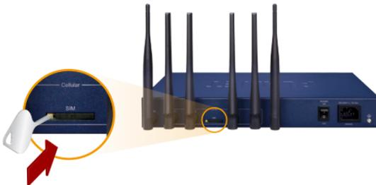
B. Pull out the tray gently from the tray slot. Place the SIM card on the tray with the gold-colored contacts facing upwards.
