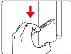
**Step 2:** Plug the RJ45 Ethernet cable into the PoE Port of the Outdoor Wireless CPE. Then, slide back the cover to finish the installation.
