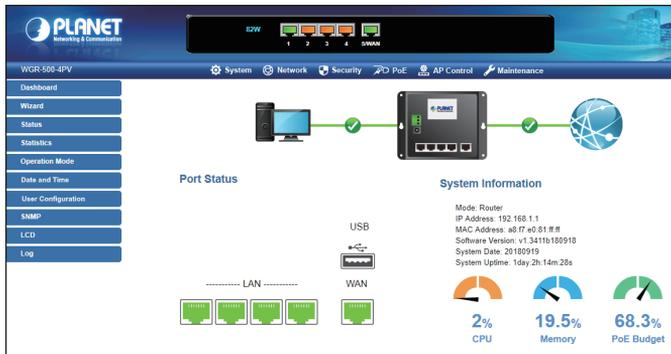
**Figure 5-3:** Web Main Screen of Industrial Router
