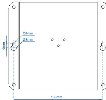
**Figure 4-2:** Getting mounting holes aligned
