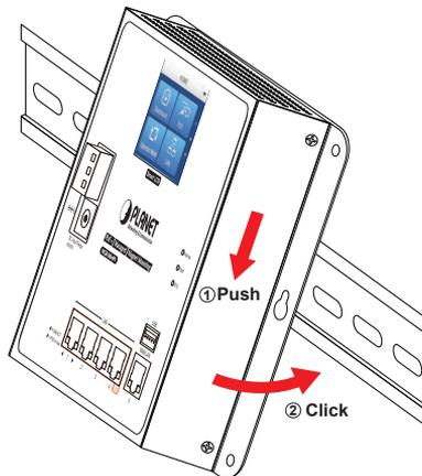
**Figure 4-6:** Router is placed on the track
