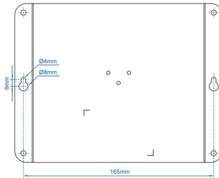
**Figure 4-1:** Getting mounting holes aligned
