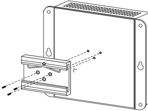
**Figure 4-5:** DIN-rail bracket is attached to router
