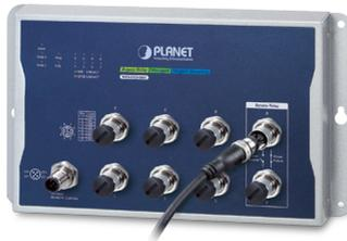
**Step 3:** Turn clockwise to tighten the cable of the M12 connector and make sure the connection is tight.
