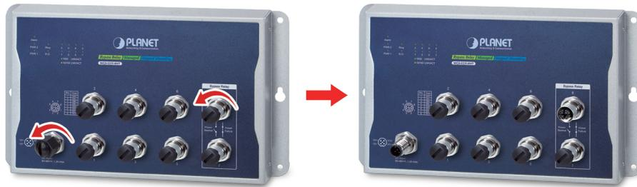
**Step 2:** Insert the M12 UTP male connector into the M12 female Gigabit Ethernet port of the Wall-mount Managed Switch.
