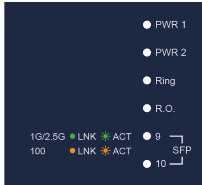
Figure 2-1-2: LED Panel of WGS-5225-8UP2SV
