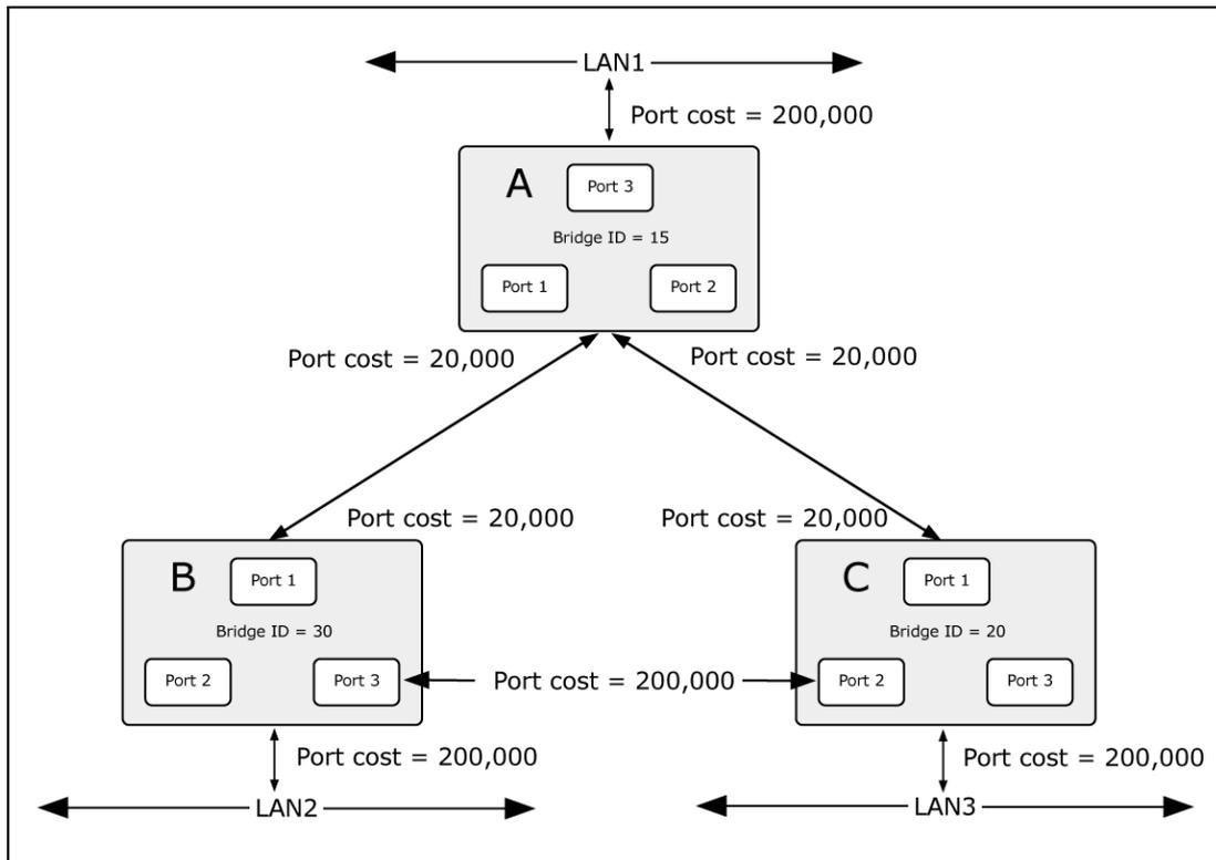
**Figure 4-3-4-2:** Before Applying the STA Rules
