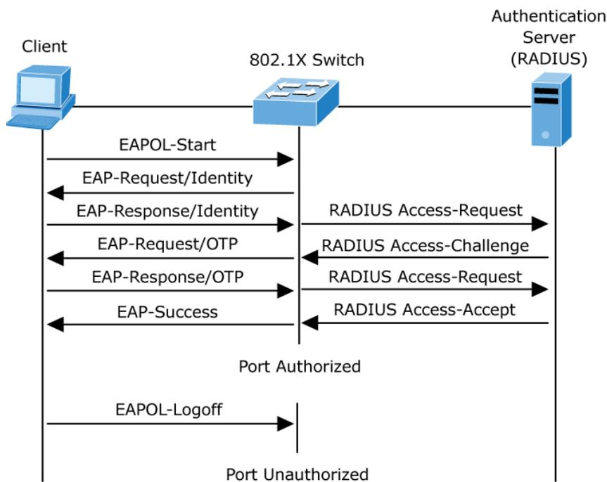
**Figure 4-5-2-2: EAP Message Exchange**
