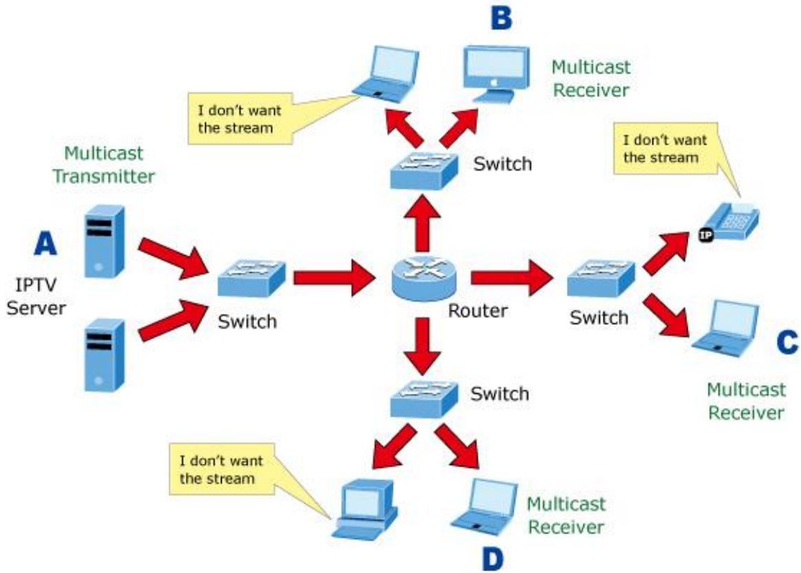
Figure 4-3-5-2: Multicast Flooding
