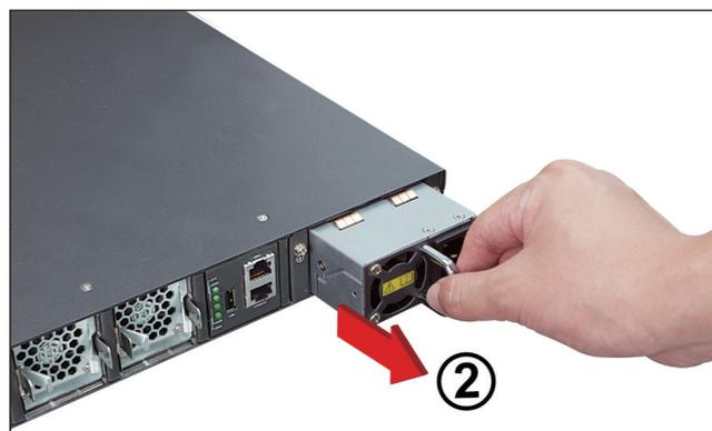
**Figure 3-3:** Removing the Power Supply Unit
