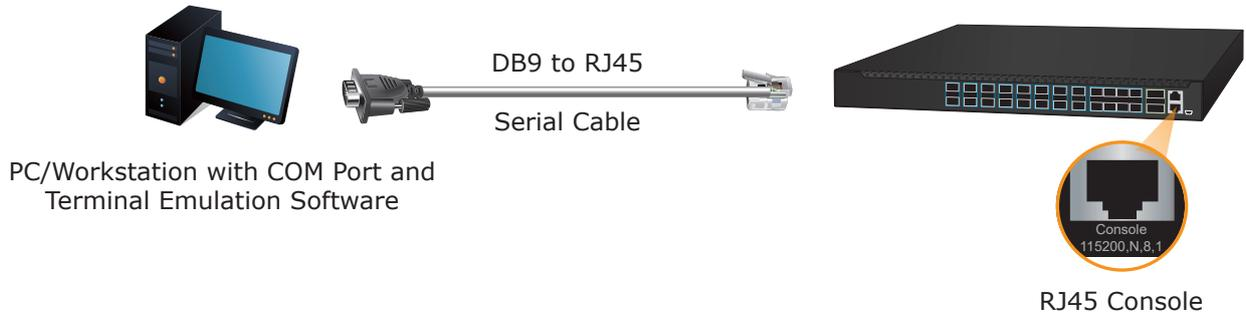
**Figure 5-1:** XGS-PON OLT Console Connectivity
