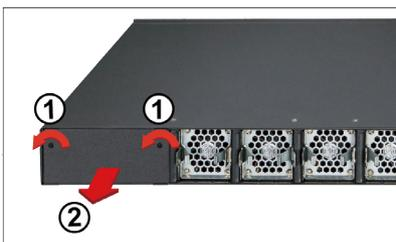
Figure 3-1 Removing the Blank Plate
