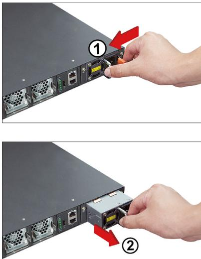
Figure 4-1 Removing the power supply unit
