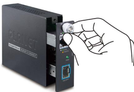
**Step 2:** Remove a blank faceplate from an empty expansion slot on the front of the chassis. The Smart Media Converter board can be installed in any expansion slot.
