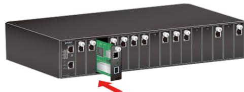
**Step 4:** Secure the Smart Media Converter board to the chassis by tightening the thumbscrew.
