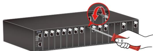
**Step 3:** Slide the Smart Media Converter board into the expansion slot, aligning it with the guide rails, until it firmly connects to the chassis' backplane.
